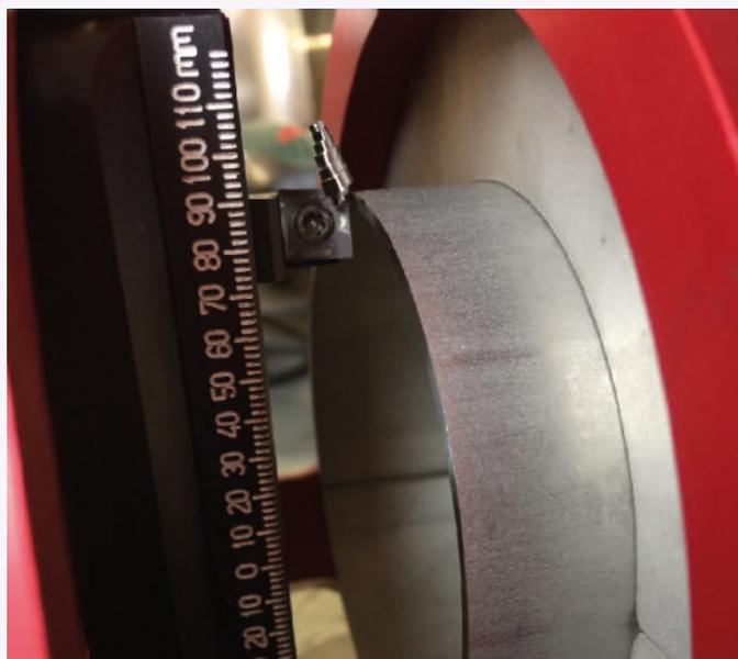
Tube with small diameters <math>< 25.4\text{ mm}</math> are particularly concerned by the facing process. They are often cut with tube cutters or abrasive cutting machines. Generally speaking, tube must be faced before welding in order to obtain quality welds.
