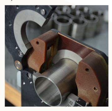
Closed heads provide optimum gas protection (closed chamber) which results in welds with very limited colouration. They are recommended for welding stainless steel tubes of wall thickness <3 mm in simple fusion without added wire.
